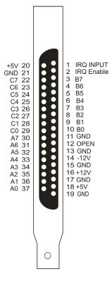
Figure 2-1. PCI-DIO24 board connector pin out
